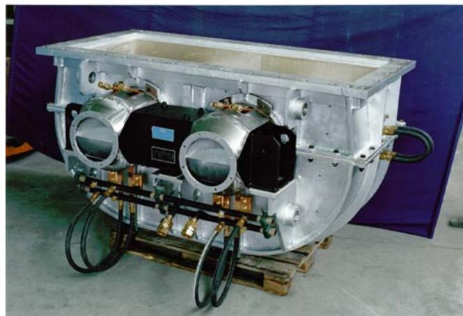
**Figure 7.** Channel inductor (nominal ratings; 500 kW, 550/620 V, 50/60Hz, system Marx)
