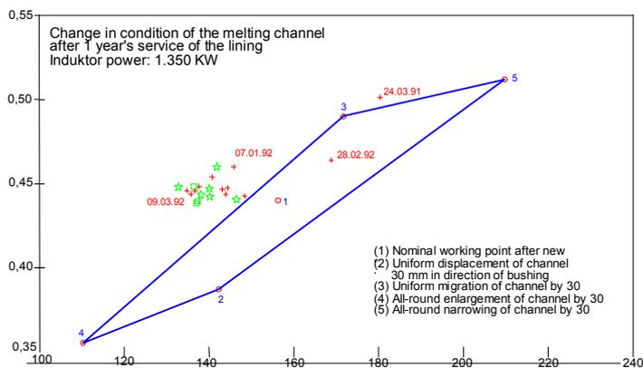
**Figure 5.** Wear diagram for inductor and channel
