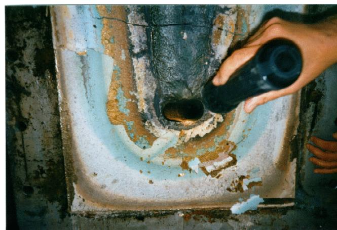
**Figure 8.** Channel condition after 14 months operation (side channel)
