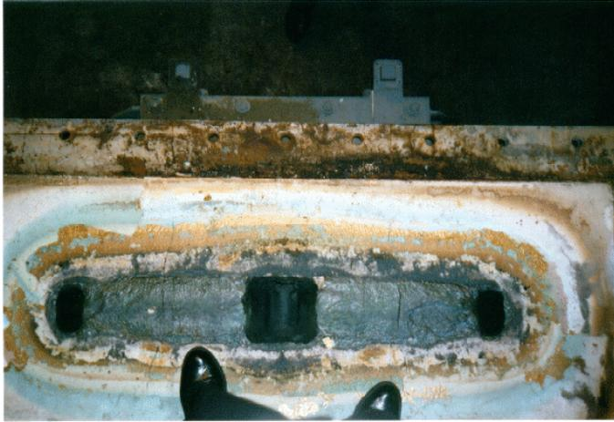
**Figure 9.** Channel condition after 14 months operation (side and middle channel)
